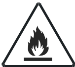
Caution: Risk of fire
